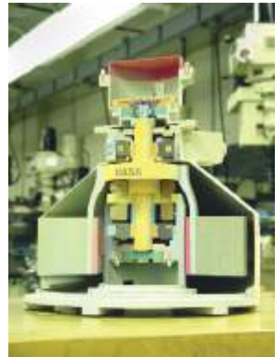
A three-dimensional printing of the output of an AutoCAD model of a NASA flywheel.
